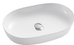
Art Basin CL-1373 Size: 615x415x135mm Vitreous china Above counter mounting
