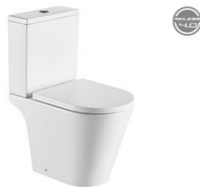
Two-piece Toilet AB-1363B • Flushing Principle: Washdown • Drainage Patterns: S-trap 250mm • Size: 590x365x790mm • Optional Accessories: Soft-closing seat cover
