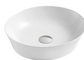
Art Basin CL-1472 Size: 400x380x105mm Vitreous china Above counter mounting
